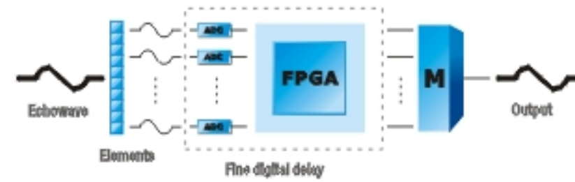
Accurate beam forming and signal processing, digital image acquisition and processing ensure images with clear-cut edge and no distortion.
